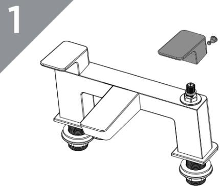
1 Remove the cap and loosen the grub screw. Remove the handle.
