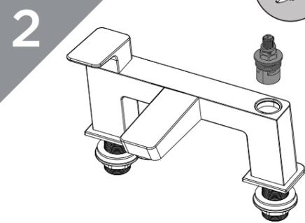
2 Remove any O-rings, soak the valve in de-scaler and wash off in clean water. Examine all seals and replace if needed. Use WRAS approved silicon based grease on all seals.
