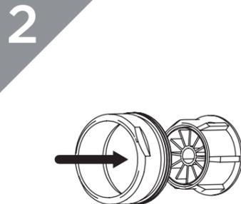
2 Separate the aerator from the collar by pushing it out of the threaded end of the collar.
