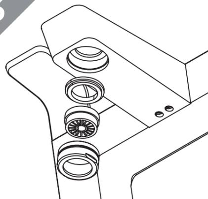
3 Replace the aerator, ensuring the washer has been fitted. Secure in place by tightening with suitable spanner.
