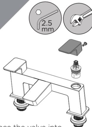
3 Replace the valve into the body and tighten in a position. Replace the handle, tighten the grub screw and push fit the cap.
