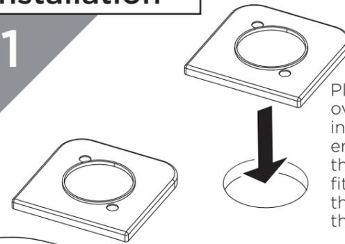
Place the plinths over the holes in the bath ensuring that the washers are fitted between the plinths and the bath.
