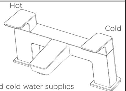
Connect the hot and cold water supplies to the threaded tails using 3/4" BSP connector (not supplied). Turn on the mains water supply letting the water flow for a few minutes to flush through the system. Check all joints and connections for any leaks.
