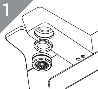
1 Loosen aerator using a spanner. Remove the aerator and the washer.
